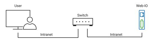
To connect to an Ethernet LAN, all you need is a free port on a switch or hub. All Web-IOs support both 100BaseT and 10BaseT, with automatic detection of the network speed.
