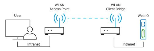
The W&T Web-IOs come shipped with a cable-connected Ethernet port for network access. A wireless LAN client bridge or a wireless access point can be used to easily incorporate Web-IOs into existing WLANs. This makes it easy to implement wireless remote control and monitoring. Additional information about WLAN integration can be found here.
