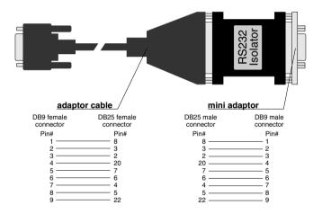
By using the short adapter cable the isolators can be connected directly to 9-pin serial devices having a SUB-D male with standard PC configuration.
