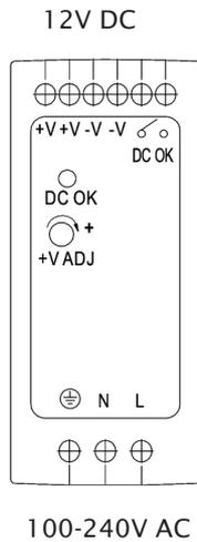
„DC OK“ indicates a potential-free contact which is closed when the output voltage is correct.
