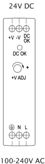
When the output voltage is correct, „DC OK“ provides a level of 24V with a load capacity of 20mA
