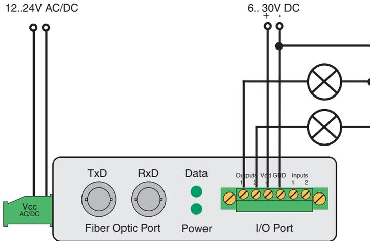
The two digital outputs of the Digital-I/O Extenders are current sourcing. The supply voltage for the outputs may be between +6 V and +30 V DC and is provided at terminals Vdd and GND.
