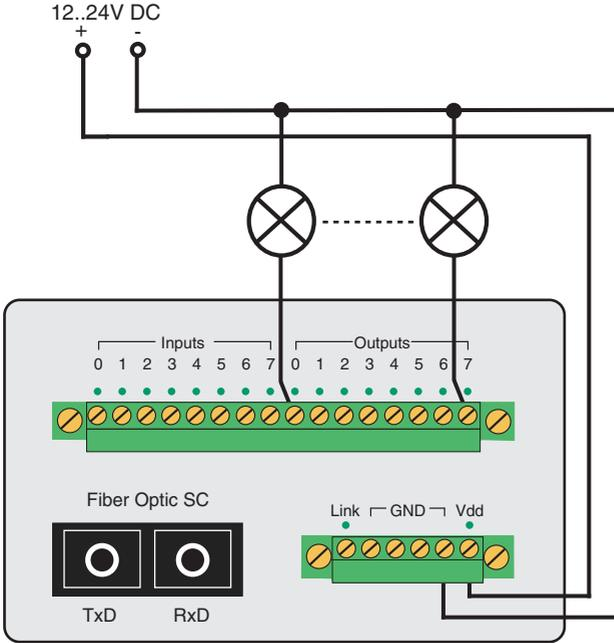
The digital outputs of the Digital-I/O Extender Sets are current sourcing and apply the voltage brought to Vdd to the output terminals. Each of the outputs can switch a maximum current of 0.5A. If loads with an inductive component (e.g. relays, contactors, solenoids etc.) need to be switched, the outputs must be additionally protected using recovery diodes.
