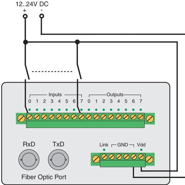
The digital inputs of the Digital-I/O Extender Set 17634 are „Type 3“ according to IEC 61131-2 and have a maximum input voltage of 30V with respect to the device reference ground.
