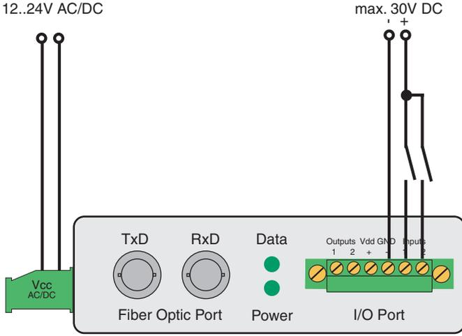
The digital inputs of the Digital-I/O Extender Set 17633 are „Type 3“ according to IEC 61131-2 and have a maximum input voltage of 30V with respect to the device reference ground.
