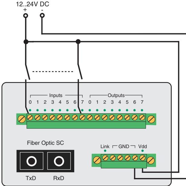
The digital inputs of the Digital-I/O Extender Set 17635 are „Type 3“ according to IEC 61131-2 and have a maximum input voltage of 30V with respect to the device reference ground.
