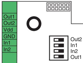
In this way each of the four channels can be configured individually as desired.
