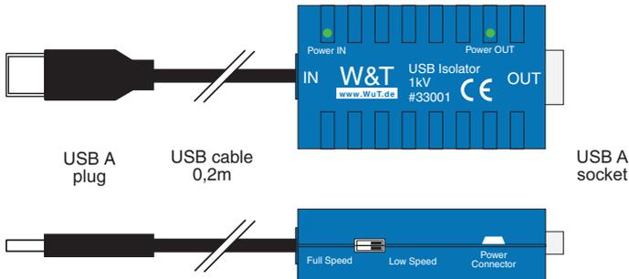
Each switch configures the upstream and downstream side of the Isolator. Since a speed conversion with the Isolator is not technically realizable, both switches must always be in the same position. The Isolator will not function with the switches in different positions.
