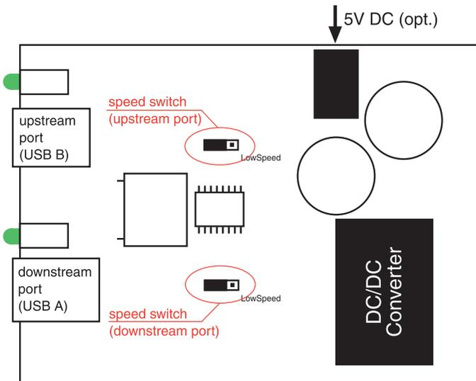
Since low speed devices are uncommon, the USB Isolator model 33204 is factory set to full speed mode.
