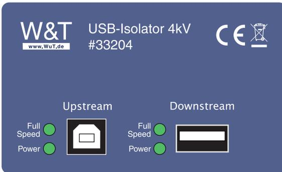
The „Power“ LED of the pair indicates correct supply voltage to the associated Isolator port, whereas the „Full Speed“ LED indicates the set speed of the Isolator.
