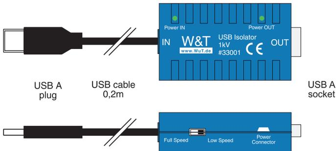
Each switch configures the upstream and downstream side of the Isolator.
