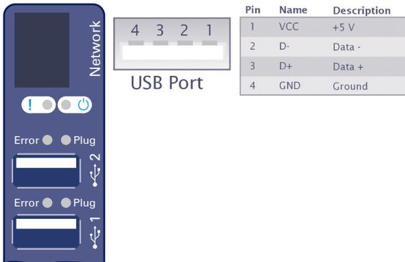
Both ports of the W&T USB-Server conform with USB 1.0, 1.1 and 2.0 with transmission speeds of 1.5 Mbit/s (Low), 12 Mbit/s (Full) and 480 Mbit/s (High). This means most USB devices using the transfer modes Control, Interrupt, Bulk and Isochronous are supported.
