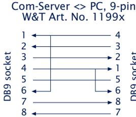
The Web-IO 1x Thermometer may only be connected via pins 2,3 and 5
