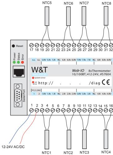
The eight NTC temperature sensors are connected to the unit as shown in the following table. The numbering corresponds to the screw terminals on the unit:
