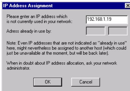
The device acknowledges the entry with an audible tone (2x/ 8x Thermometer only) and accepts the set IP address. After clicking again on the Scan button, this address is displayed in the WuTility.
