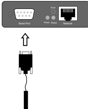
The supplied NTC probe is already preconfigured and is simply plugged into the DB9 connector in the device.
