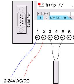
The 12-24V AC/DC supply voltage is brought to the unit on pins 1 and 2 located on the lower screw terminal block.
