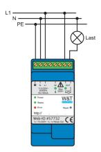
The "OUT" LED comes on when the contact is closed. Details about the load capacity of the relay contact can be found in the technical data for the Web-IO.
