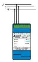
The external lead must be connected to the terminal labeled "L1", and the neutral conductor to terminal "N".
