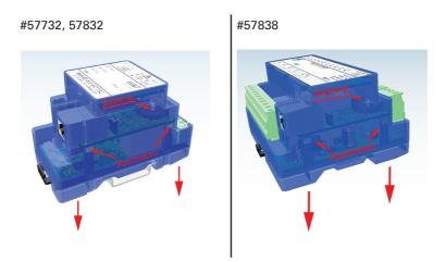
Press a pointed object against the side latch hook of the housing while pulling the base of the housing out of the top shell.
