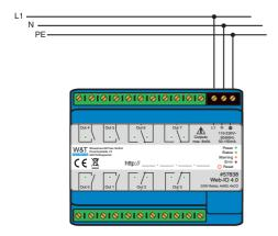
The external lead must be connected to the terminal labeled "L1", and the neutral conductor to terminal "N".
