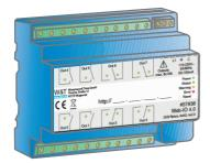
Das Web-IO 4.0 230V Relais 4xNO, 4xCO (hereinafter referred to simply as Web-IO) is powered with 230V, can monitor a 230V signal and switch a 230V load. Connections are made via screw terminals.
