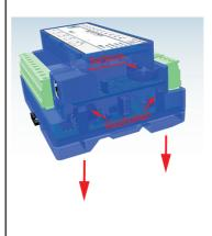
Press a pointed object against the side latch hook of the housing while pulling the base of the housing out of the top shell.
