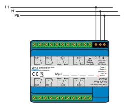
The external lead must be connected to the terminal labeled "L1", and the neutral
