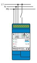
Voltages above approx. 80Veff referenced to the "N" terminal are recognized as an "ON" signal and indicated by the green "IN" LED. A switching state must be present for at least 50ms to be reliably detected.
