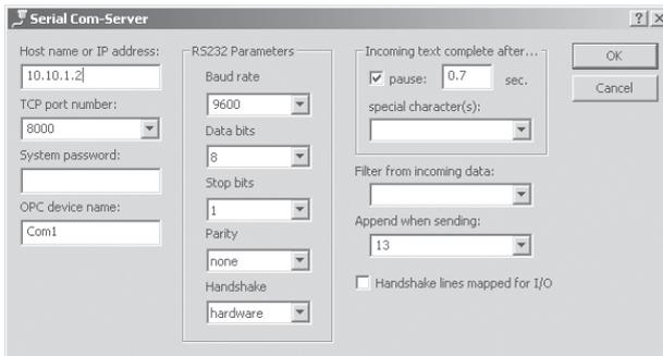
The required connection data for the Com-Server, consisting of the IP address, TCP port and system password, are entered into the corresponding fields of the following window.
