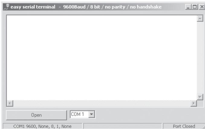
Now turn the Com-Server on and off to reset it and while it is starting up hold down the „x“ key (lower case, no Caps Lock!). After about 2-3 seconds the prompt *IP no.:+<ENTER>*: will appear in the terminal window.
