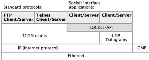
Each mode is explained individually in the following sections. The server mode does not have to be configured separately; it is activated when a client of a TCP/IP station directs a connection request to the server in the Com-Server.
