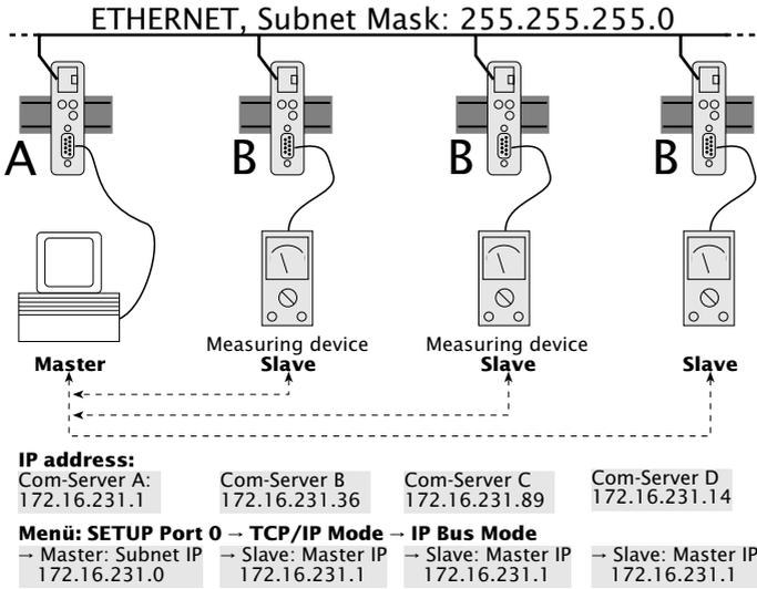
*The serial devices must send their data using their own proofing protocol. Since the Com-Servers use Internet Protocol (IP) as the network transmission protocol, they cannot ensure data integrity.*
