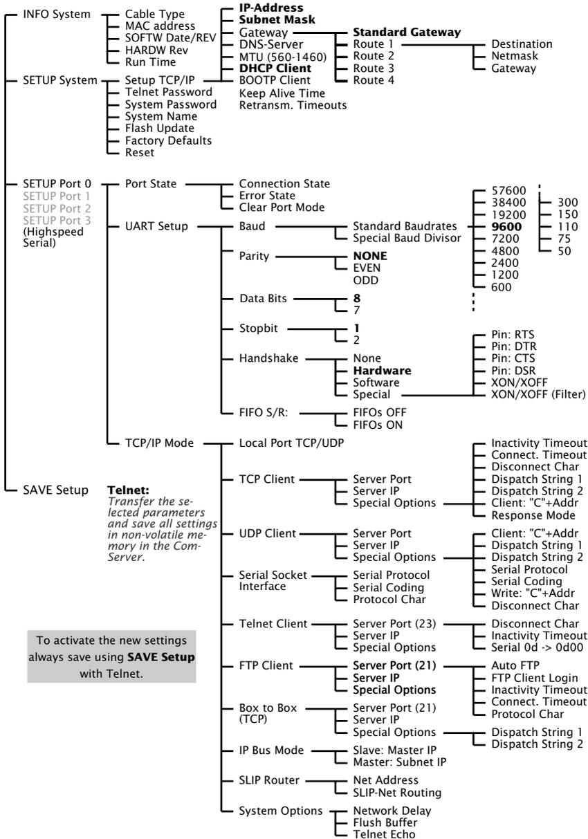
To activate the new settings always save using **SAVE Setup** with Telnet.
