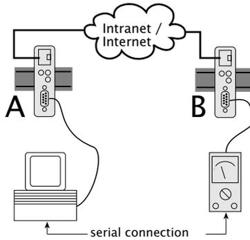
The Slave address is only configured on the Master Com-Server. The Dispatch Strings may be set on both ports however. In addition, the serial transmission parameters (baud rate, data bits, etc.) in *both* Com-Servers must conform to those of the connected devices.
