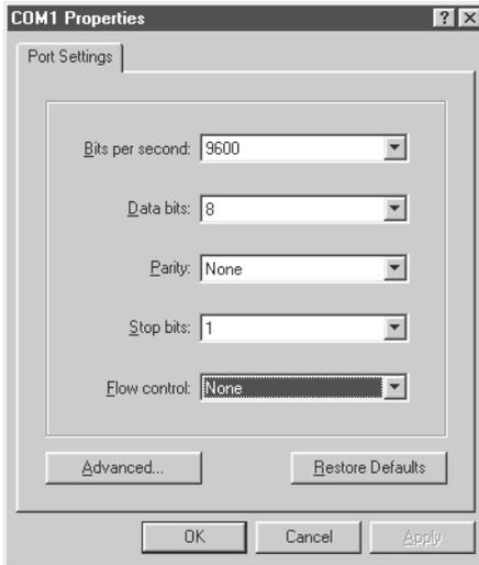
4. After you have confirmed the settings with OK, you will find yourself in the actual terminal window. All keyboard entries are output through the selected COM port. Now turn the Com-Server on and off to reset it and while it is starting up hold down the „x“ key (lower case, no Caps Lock!). After about 2-3 seconds the prompt *IP no.:+<ENTER>*: will appear in Hyperterminal.
