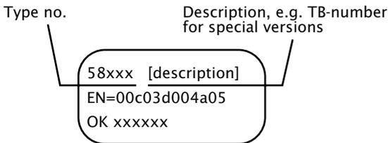
**⚠** *In particular if the sticker indicates an TB number as the part number, it is possible that the Com-Server has a special, customer-specific firmware or configuration. This would be overwritten by uploading the standard firmware. Please contact the responsible administrator in such cases before the update.*
