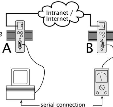
**Example 2:** A control program polls a measuring device; the measuring device can actively send data to the control program.
