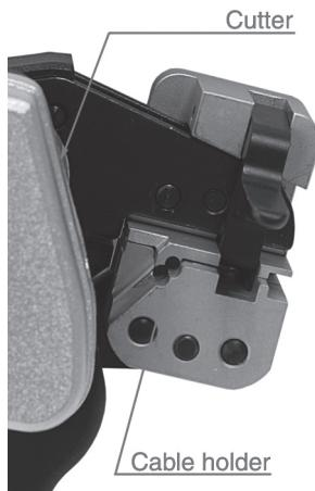
cable is securely held in the clamping block. While doing this take care not to squeeze the grips until they touch, since this will release the plier again.
