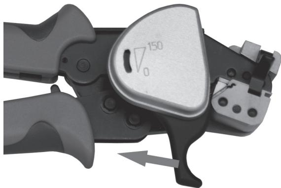
A firm pull with the index finger quickly and cleanly cuts the fiber optic cable. To remove the cable from the clamping block, open the plier.
