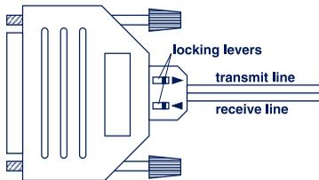
Please note that when connecting two fiber optic components, the emitter of the first must always be connected to the receiver channel of the second component.
