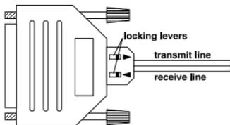
Please note that when connecting two fiber optic components, the emitter of the first must always be connected to the receiver channel of the second component.
