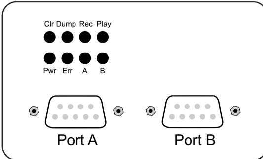
**Configuring the serial ports and Buffer operating modes requires opening the housing of the device. For this purpose it is advantageous to screw a SUB-D plug with body to one port on the Buffer and use the attached plug to assist in pulling off the housing cover.**
