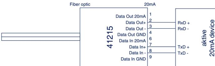
**Interface Tx loop active, Rx loop passive**
