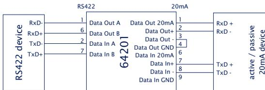
RS485 <-> 20mA, interface Tx loop active, interface Rx loop passive
