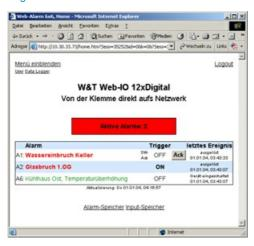
This device makes it possible to use sensors with switching contacts as initiators for alarm events. The alarm can be triggered either when single events occur or when a defined pulse count is reached on the respective input. Messaging can take place locally through switching of the digital outputs and be forwarded in the form of e-mail, SNMP trap, UDP and TCP client, syslog messages and FTP over a TCP/IP based network.
