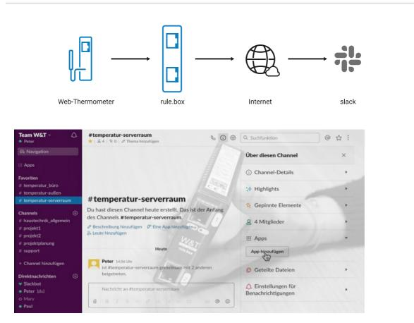
Get the overview from remote locations - with rule.box and Node-RED in just four steps. Take a look at the video shown here or read the step-by-step guide at the bottom of this page.
